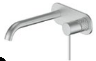
Wall Basin Mixer w/ faceplate 1830252160 | Brushed Brass 1830252170 | Matte Black 1830252130 | Brushed Stainless 1830252190 | Gun Metal WELS 5 Star 6.0L/M | MP | Fixed Spout 180mm | European Brass Cartridge
